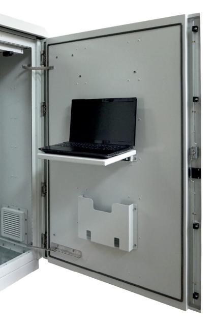
A PU-foam seal in combination with a unique 4-point locking system ensures the appropriate compression and seals the housing perfectly, so that the IP66 degree of protection is achieved. Other installations can be flexibly fixed to the vertical and horizontal system profiles. Further system profiles can be easily and conveniently ordered and subsequently retrofitted.
